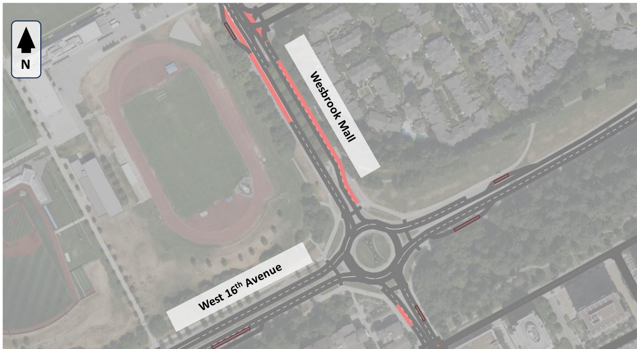
Figure 6.7: Coding of bus-only lane on Wesbrook Mall between Thunderbird Boulevard and West 16 th Avenue
