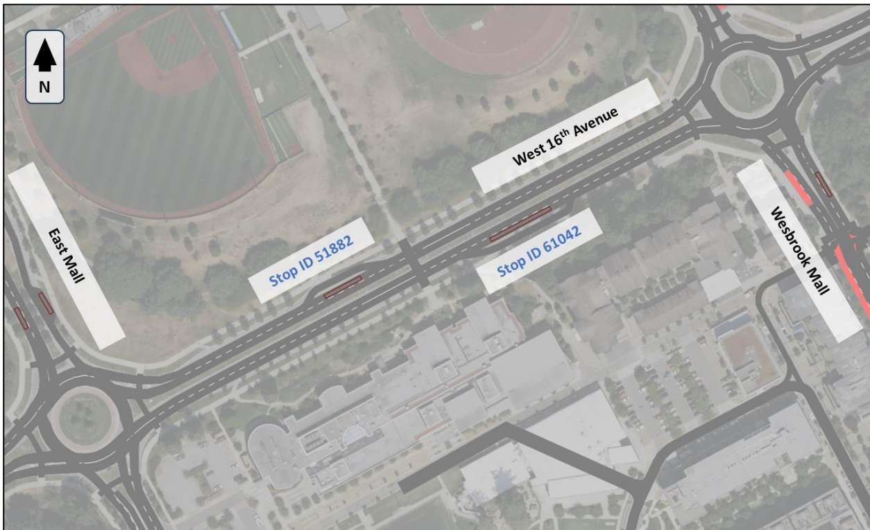
Figure 6.5: Coding of in-lane bus stops along West 16 th Avenue between East Mall and Wesbrook Mall
