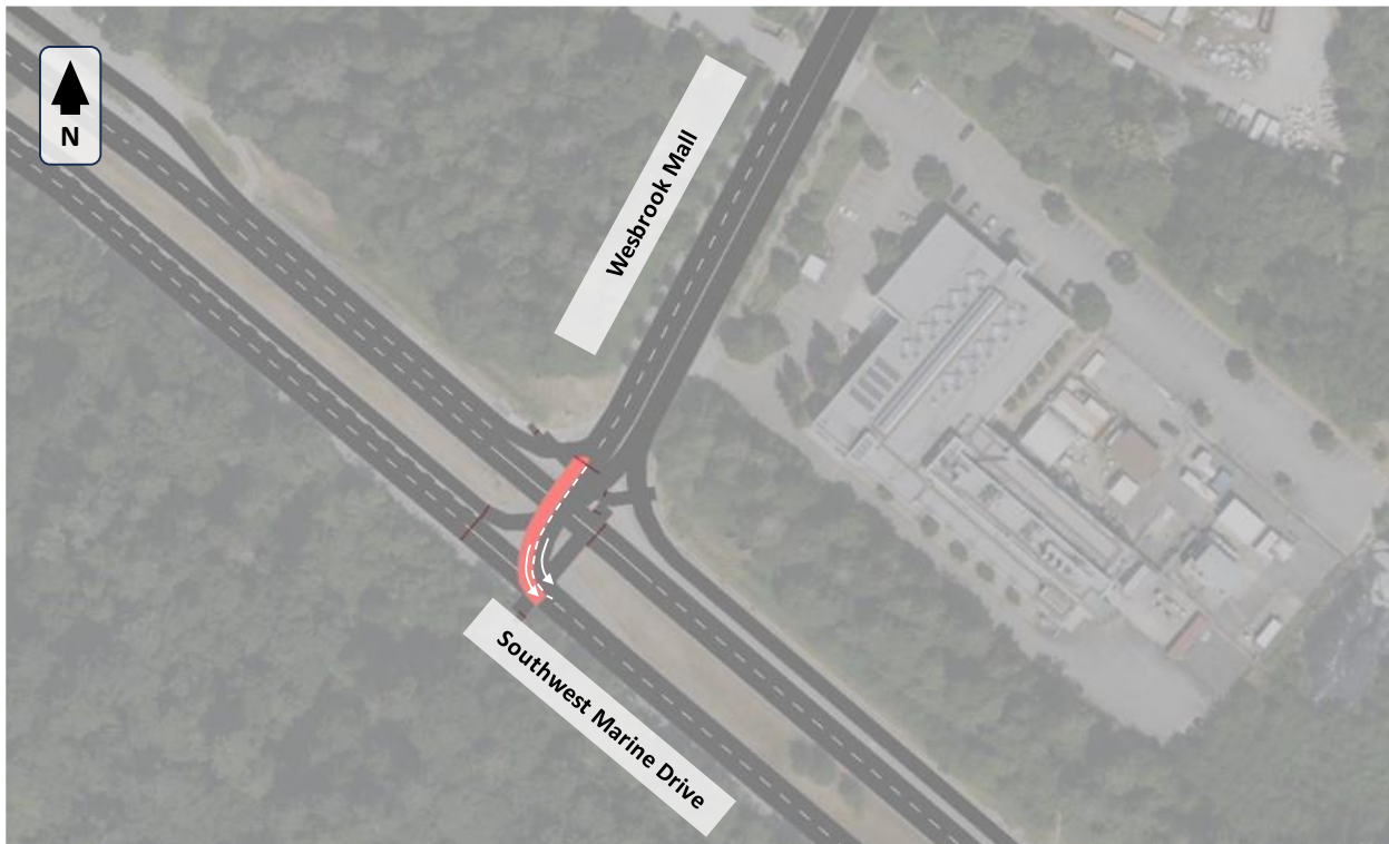
Figure 6.6: Coding of additional lane along southbound Wesbrook Mall at Marine Drive
