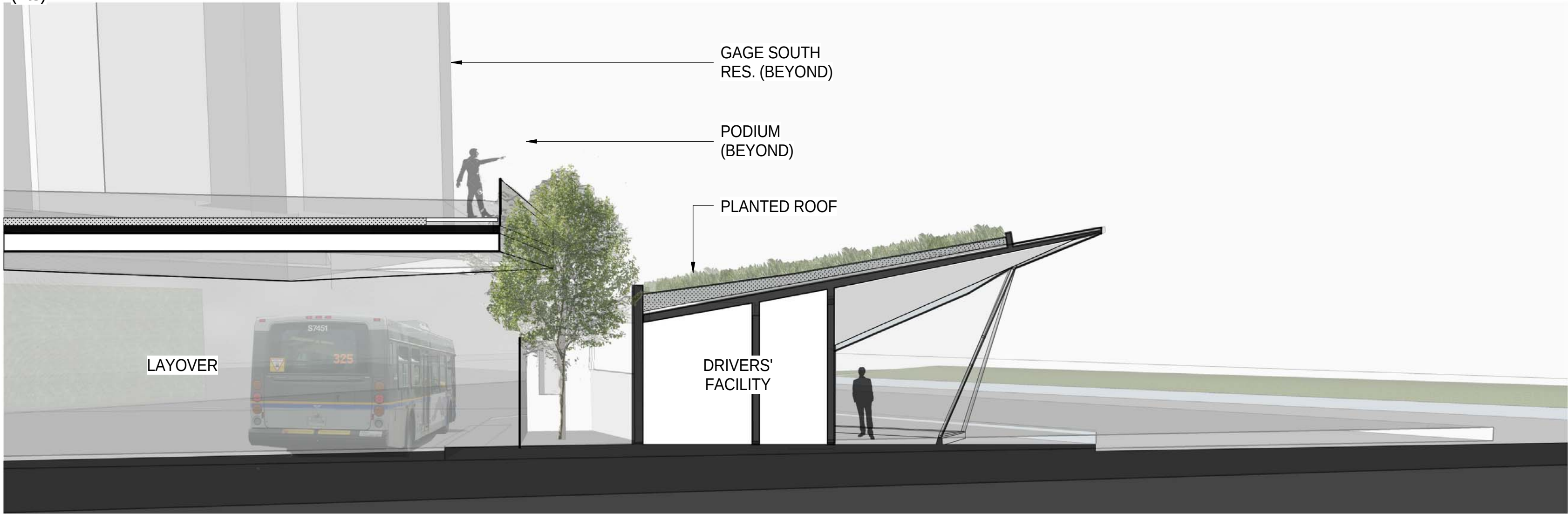
5. DRIVERS' FACILITY - NORTH-SOUTH SECTION (nts)
