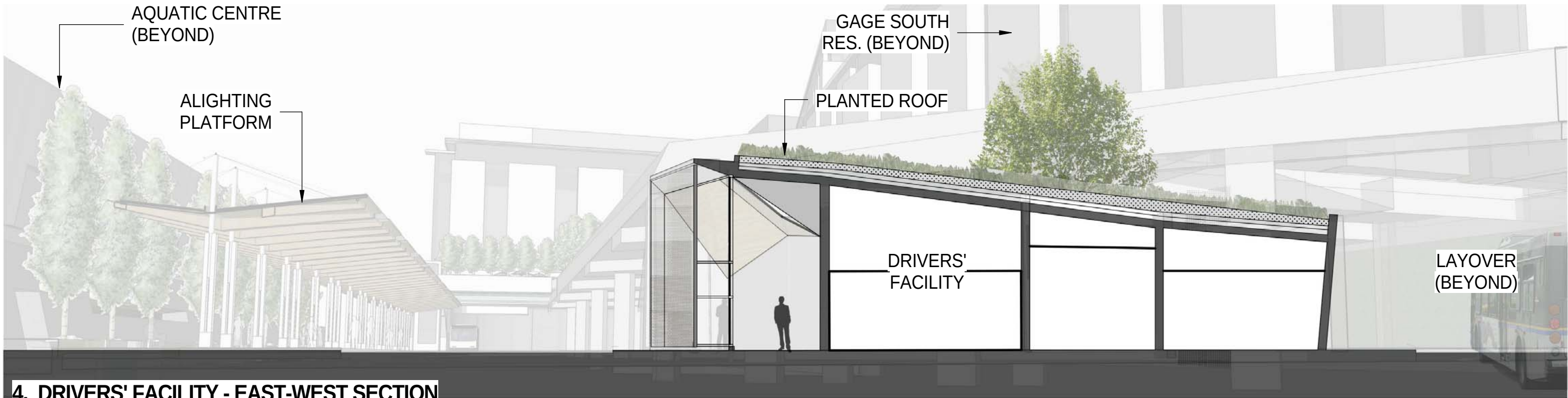
4. DRIVERS' FACILITY - EAST-WEST SECTION (nts)
