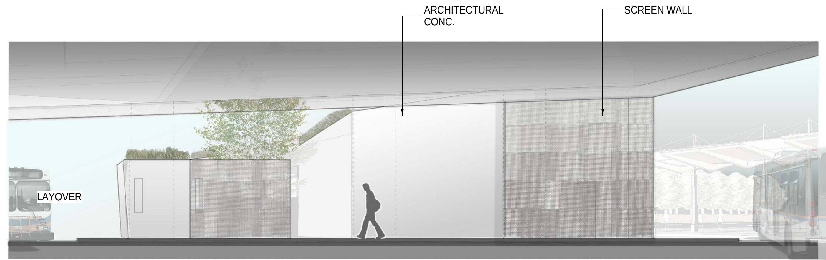
1. DRIVERS' FACILITY - NORTH ELEVATION (nts)
